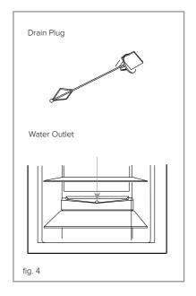
The water drain hole at the back of the fridge compartment and the evaporating tray should be cleaned periodically to prevent the defrosted water from collecting inside the fridge compartment. The drain plug can be used to clean the drain hole.
