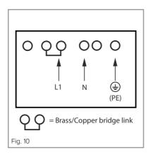
Ensure that the brass links are securely fitted. Failure to do so may prevent the hob from operating correctly.
