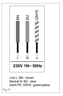
This appliance is intended to be connected to fixed wiring by a double pole switch, having a contact separation of at least 3mm in all poles. The switch must be positioned no further than 2m from the appliance.
